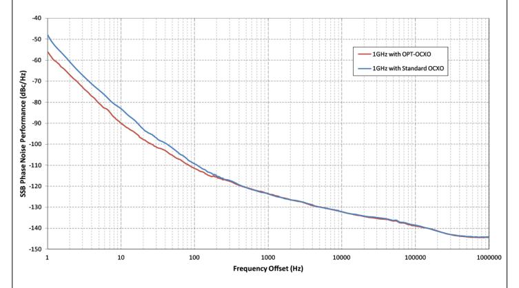
Figure 5: SSB Phase Noise OPT-OCXO Comparison (Pout=+10dBm)
