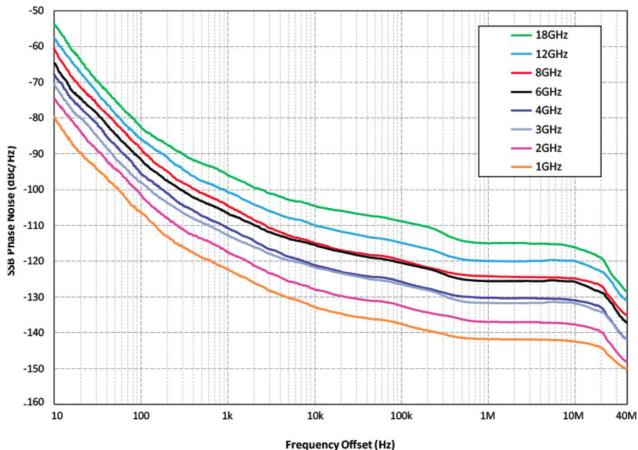
Figure 4: SSB Phase Noise (Pout=+10dBm)
