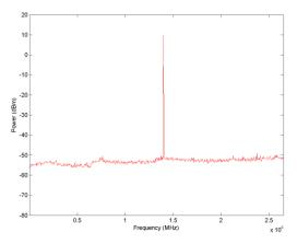
Figure 12b: 14GHz Broad Band Spectrum
