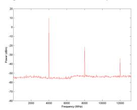
Figure 8b: 4GHz Broad Band Spectrum
