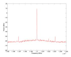
Figure 11a: 12GHz Narrow Band Spectrum
