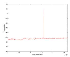
Figure 13b: 16GHz Broad Band Spectrum
