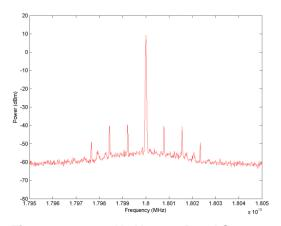
Figure 14a: 18GHz Narrow Band Spectrum
