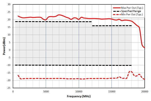
Figure 1: Maximum and Minimum Amplitude Threshold
