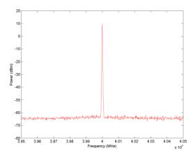
Figure 8a: 4GHz Narrow Band Spectrum
