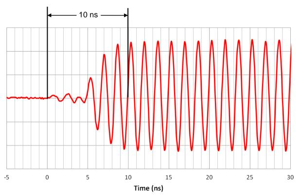
Figure 3: External Pulse Modulation Rise Time (seconds)
