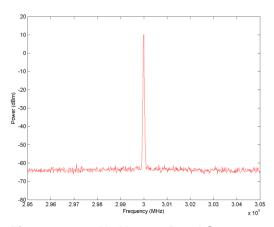
Figure 7a: 3GHz Narrow Band Spectrum
