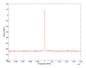
Figure 6a: 1GHz Narrow Band Spectrum
