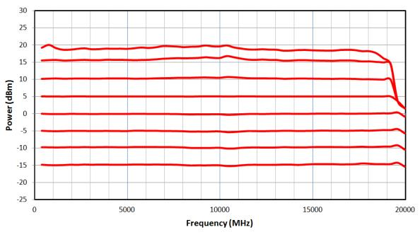
Figure 2: Calibrated Output Power Accuracy vs. Frequency
