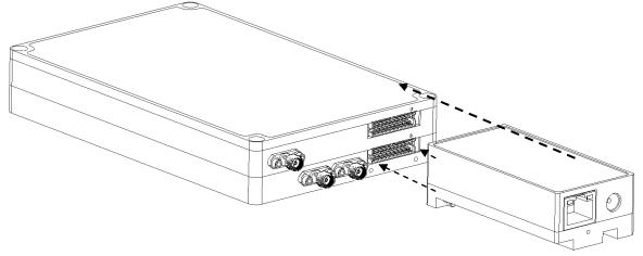
Each variation of the HCM Communications Module securely fastens to the synthesizer and comes complete with an AC power supply and the appropriate cable. HCM modules are a recommended accessory as the first step in integrating the HSM series synthesizers via the SPI bus. More information is available upon request.
