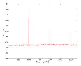
Figure 6b: 1GHz Broad Band Spectrum
