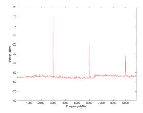
Figure 7b: 3GHz Broad Band Spectrum
