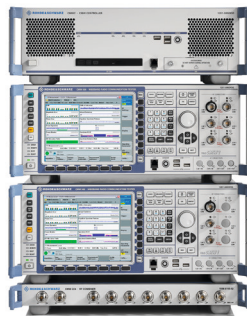
R&S®CMWflexx RF and protocol testing for LTE-A, e.g. 4 DL CA up to 8x2 MIMO, including internal fading
